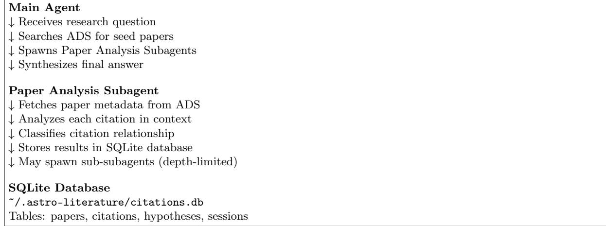
**Figure 1.** Architecture of the recursive literature analysis system.
